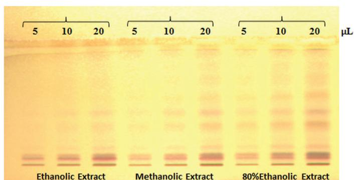
**Fig 1.** RP-TLC chromatogram of ethanol, methanol, and 80% ethanol extracts of the aerial part of *A. annua* detected under visible light after spraying with FBS and intensification by spraying with 10% NaOH.
