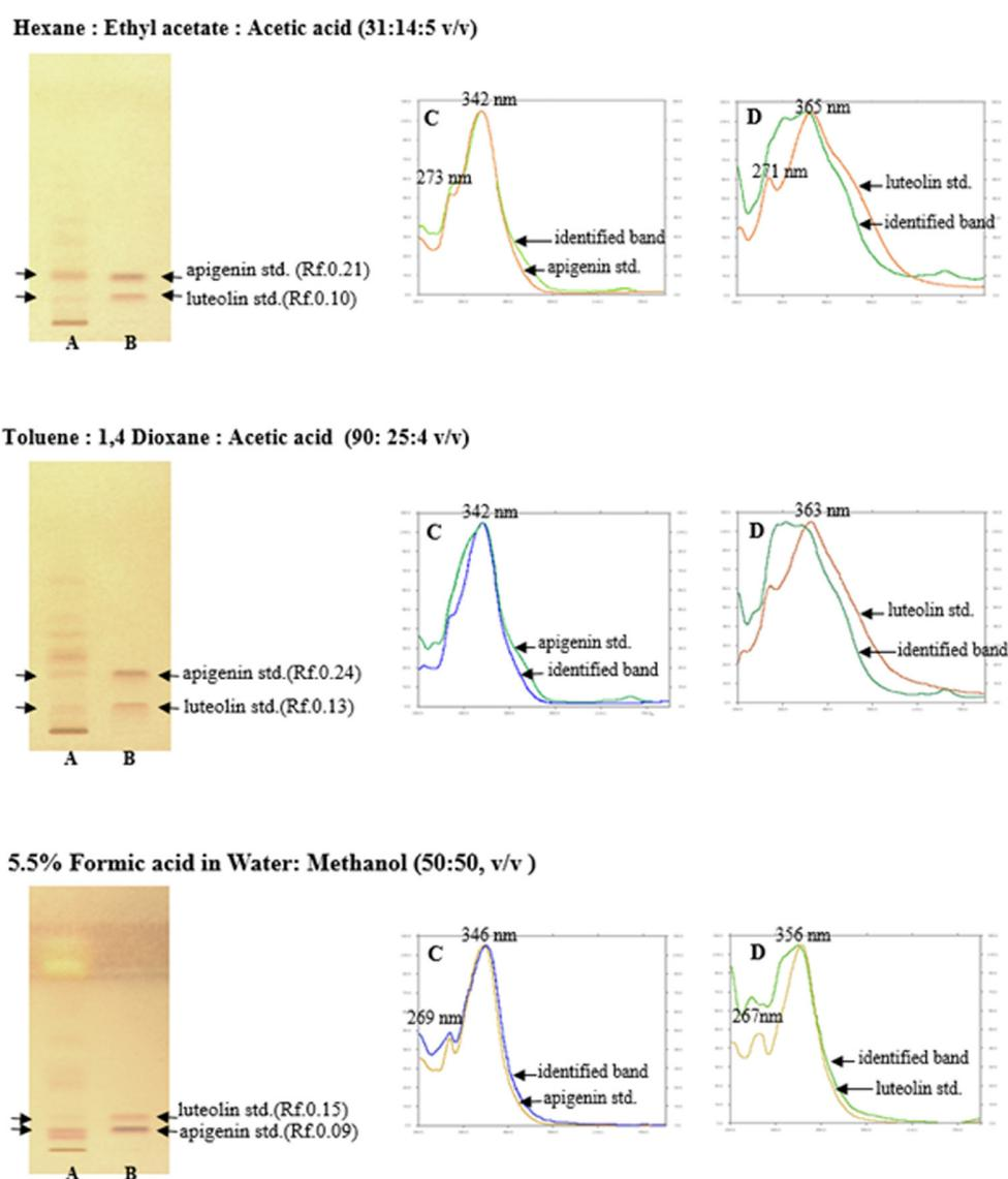
**Fig 4.** Detection of apigenin and luteolin in *A. annua* under visible light after spraying with FBS and intensification with 10% NaOH in 3 condition systems: A) 80% ethanolic extract of *A. annua*; B) mixed marker solution; C) absorbent overlay of apigenin marker along with the sample; and, D) absorbent overlay of luteolin marker along with the sample.
