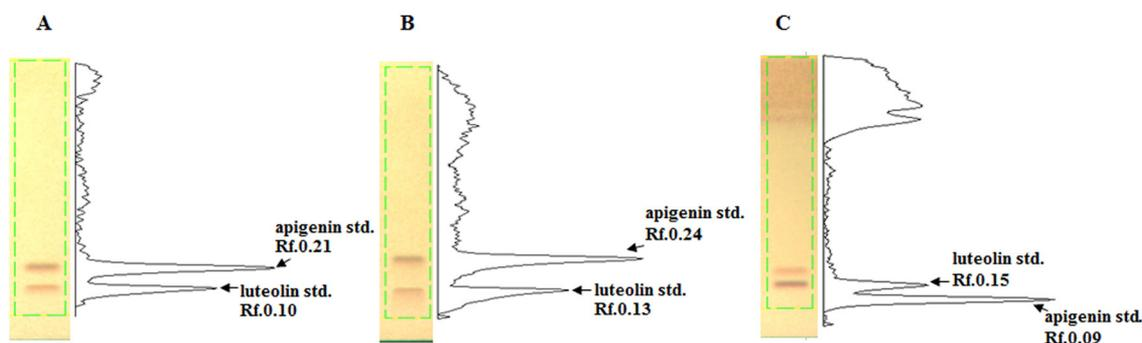
**Fig 3.** Chromatograms of apigenin and luteolin in a mixed marker solution developed in a NP-TLC plate with A) hexane : ethyl acetate : acetic acid (31:14:5, v/v); B) toluene : 1,4-dioxane : acetic acid (90:25:4, v/v); and, C) in an RP-TLC plate with 5.5% formic acid in water : methanol (50:50, v/v). Bands were detected under visible light after FBS staining.
