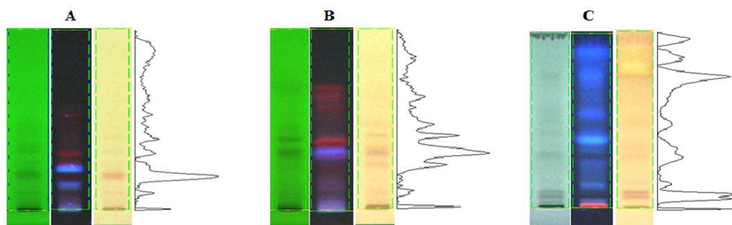
**Fig 2.** Chromatogram fingerprint of *A. annua* developed in a NP-TLC plate with A) hexane : ethyl acetate : acetic acid (31:14:5 v/v); B) toluene : 1,4-dioxane : acetic acid (90:25:4, v/v); and, C) in an RP-TLC plate with 5.5% formic acid in water : methanol (50:50, v/v). Visualization was performed under UV light (254 and 366 nm) and visible light after spraying with FBS.
