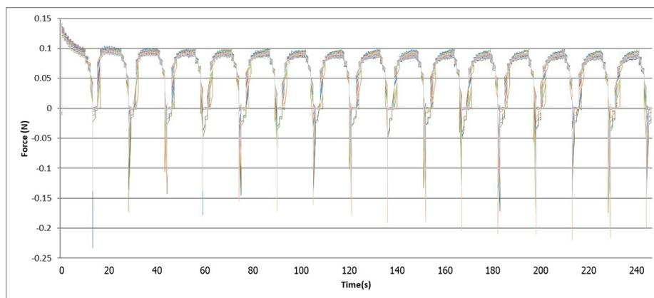
**Fig 4.** Forces of 16 consecutive loading, unloading, and resting pattern of prototype monofilaments put in controlled condition with fixed humidity at 45%.
