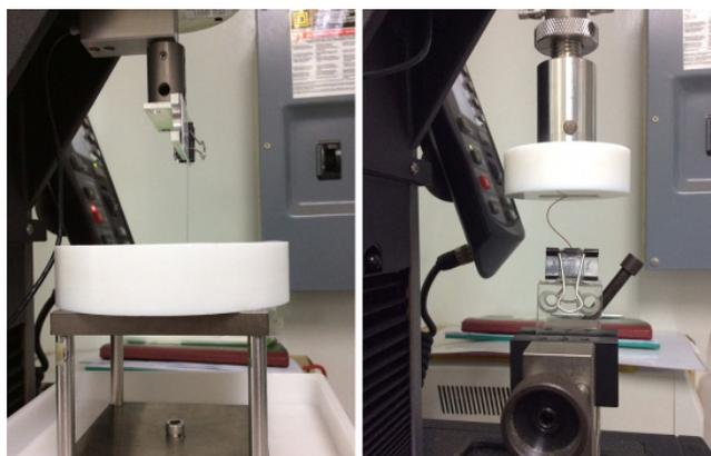
**Fig 1.** Commercial monofilament (left) and prototype monofilament (right) on a universal testing machine for compression test to simulate sensation testing on the patient's foot.
