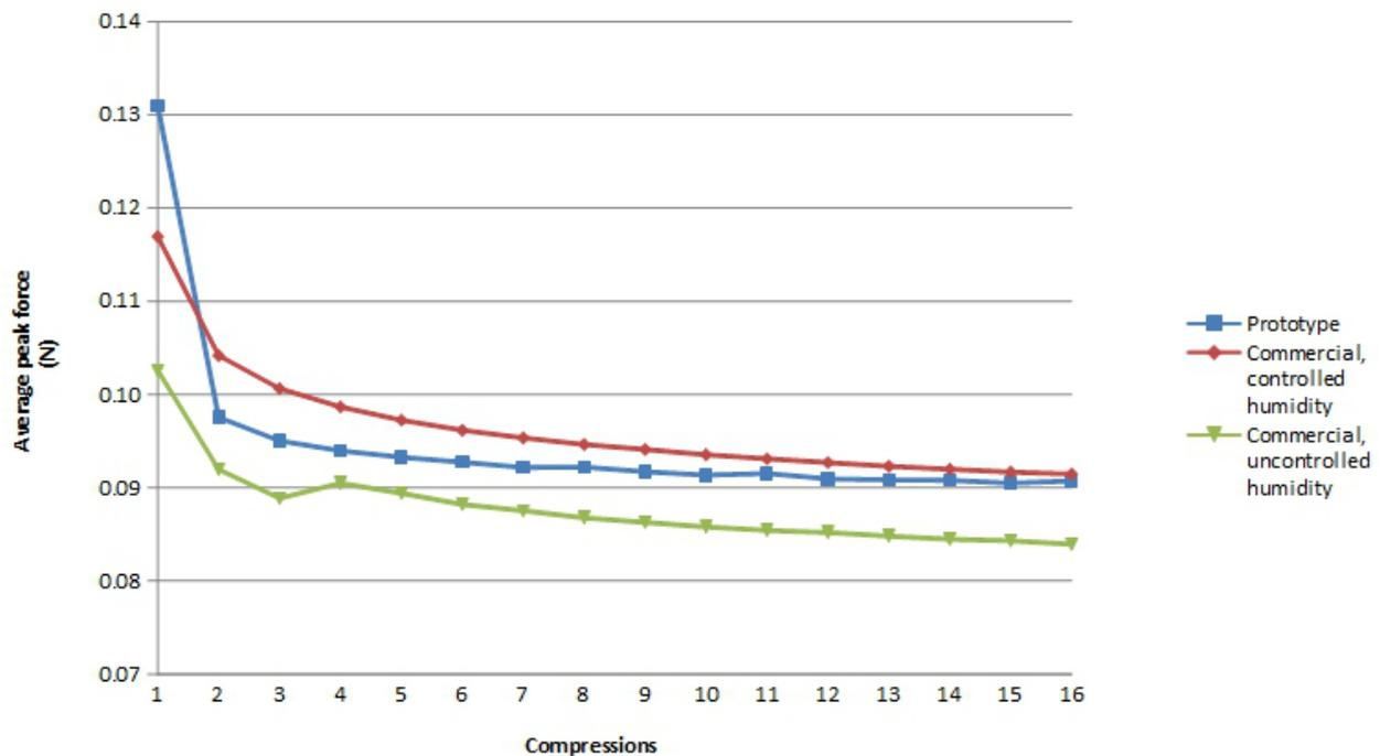
**Fig 5.** Average peak forces of commercial monofilaments in both indoor humidity condition and controlled condition with fixed humidity at 45% and prototype monofilaments in controlled condition with fixed humidity at 45% after 16 consecutive compressions.
