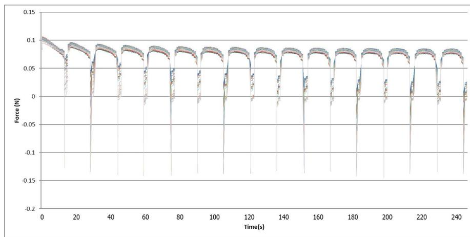
**Fig 2.** Forces of 16 consecutive loading, unloading, and resting pattern of commercial monofilaments put in indoor humidity condition.
